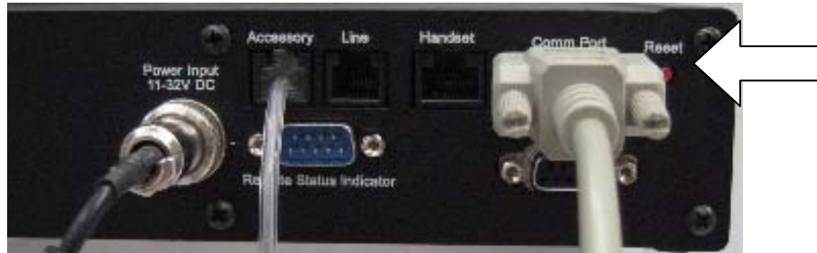
Figure: Serial cable connected to Comm Port
